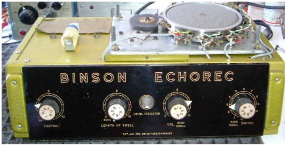
Figure 23.1: Binson Echorec used an electrostatic drum for delay
